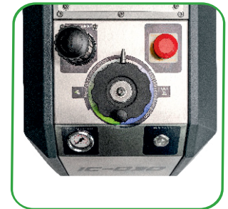
DRY ICE CONSUMPTION CONTROL PANEL
